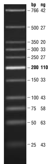
Quick-Load LMW DNA Ladder visualized by ethidium bromide staining on a 1.8% TBE agarose gel. Mass values are for 0.5 µg/lane.
