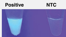
Visualization using a fluorescent intercalating dye (e.g., ethidium bromide, SYBR® green or calcein/HNBlue)
